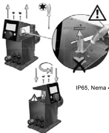
Fig. 7 Adjusting control cube
